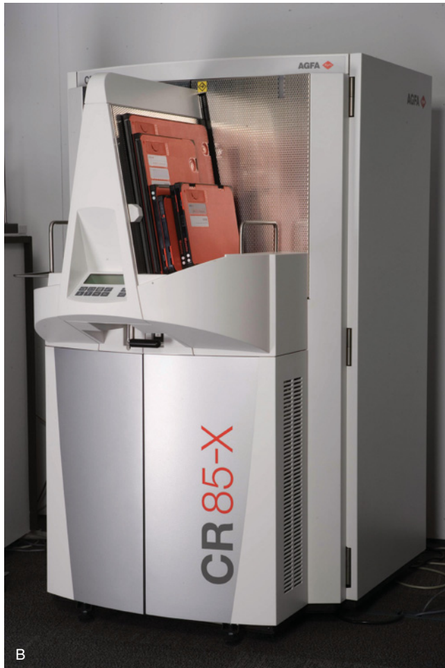
Figure 4.1. (A and B) Single- and multiple-plate computer radiography reading units. Used with permission from Agfa HealthCare Corporation, Copyright 2009. All rights reserved.
