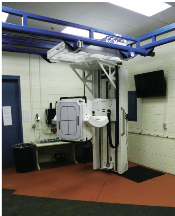
Figure 4.53. The gamma camera is mounted on a lift system with a yoke to move the camera in different directions. Both cameras can be positioned anywhere around the horse using a track system. Courtesy of Alejandro Valdés-Martínez.
