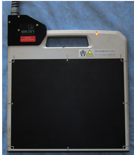
Figure 4.2. Direct flat panel detector (9 × 11 inch imaging area). Courtesy of Alejandro Valdés-Martínez.
