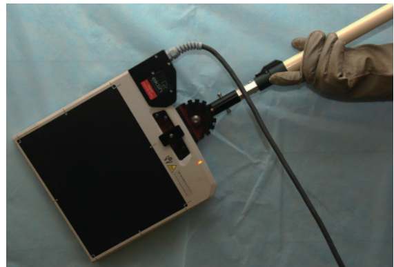
Figure 4.5. Direct flat panel detector with handle attached. Courtesy of Alejandro Valdés-Martínez.
