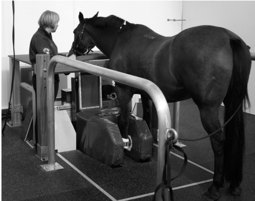
Figure 4.65. The Hallmarq Equine Limbscanner® (Hallmarq Veterinary Imaging, Guilford, UK) is an open, low-field magnet, mounted vertically at floor level that allows MRI to be performed on standing, sedated horses. Courtesy of Michael Schramme.
