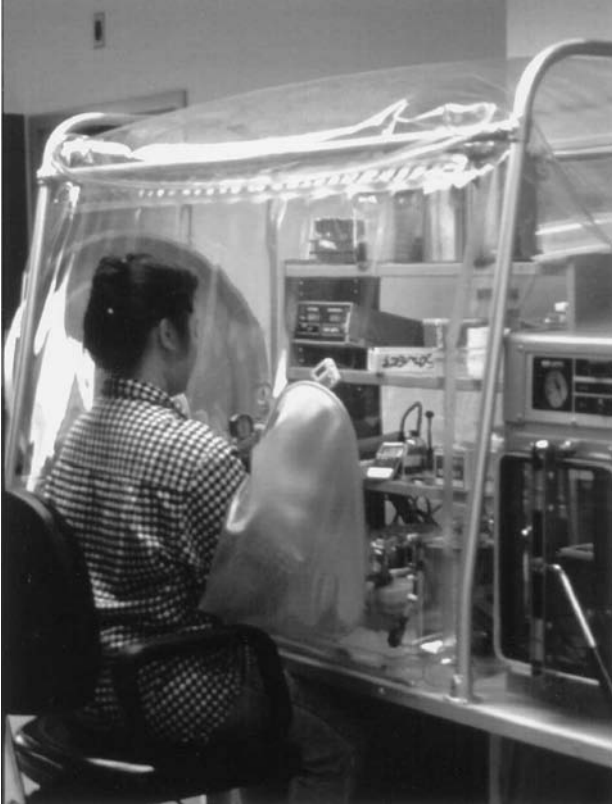
FIGURE 57.2 Anaerobic glove box used for growing methanogens. Materials are introduced into the glove box through an airlock located on the side.
