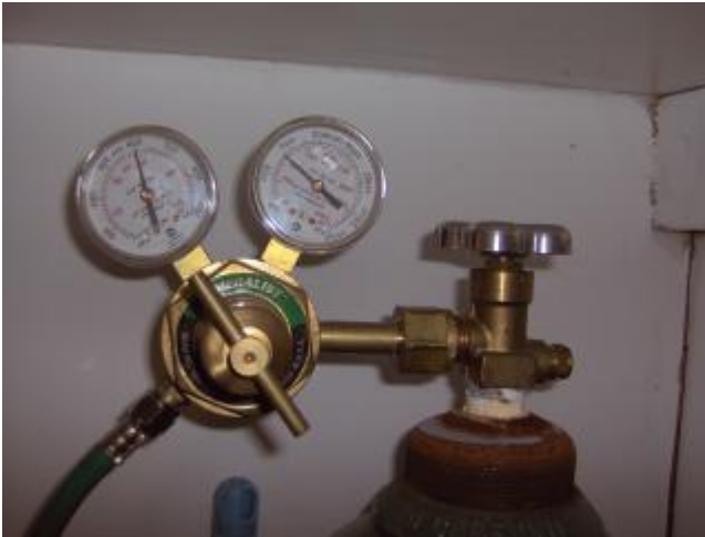
Figure 8.1. Oxygen tank regulator with the gauge on the right indicating tank pressure and the gauge on the left indicating line pressure.
